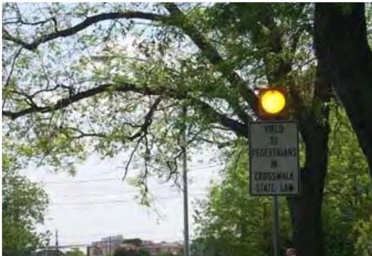
Flashing yellow beacon light used to signal drivers of a bike/pedestrian crossing.
